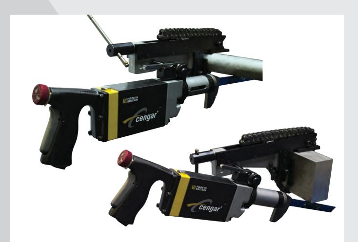
A more powerful version of the CL75 saw and is suitable for cutting all types of steel section and pipes up to 150mm (6") diameter. The CS75 can be used freehand as well as being fitted to a standard clamp or power feed clamp for square cutting.
