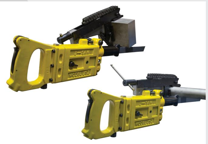
The JSZ is primarily used in the Oil, Gas and Petrochemical and Pipe Fabrication Industries for cutting steel sections and pipe up to 300mm (12") diameter. The Saw uses 25mm (1") Bi Metal blades, comes complete with a pipe & profile clamp and a blade guide to ensure straight cuts. This dual speed Saw is fitted with automatic lubrication and a trigger lock and using it in a mounted position dramatically reduces vibration.
