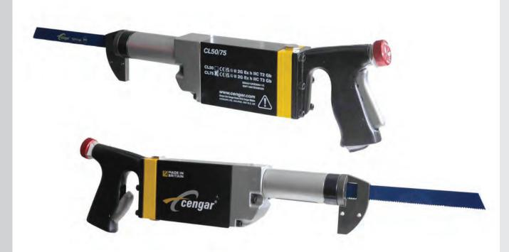
The CL75 saw uses 19mm (3/4") wide Bi Metal blades to cut pipes including stainless steel and cast iron up to 150mm (6") diameter. It can also be fitted to a standard or power feed clamp for square cutting.
